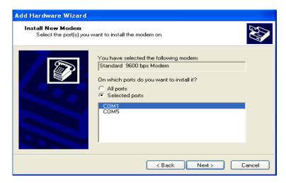
Select COM port to which modem is connected as shown above and press Next>
